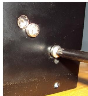
If required despite manufacturing adjustment, you can adjust the alpha angle and the vertical position of the spectrum on the CCD camera by using the two large screws on the side of the spectrograph. Be very careful as the adjustment is very sensitive.
