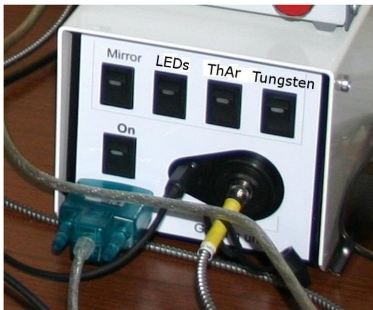
Fig: front of the calibration unit with RS232 serial cable, mirror control cable and 200µm calibration fiber
