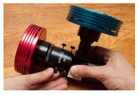
It is probable that the slit direction will have moved : rotate the guiding camera to put it back horizontal. If required, re-focus the slit image in this position.
