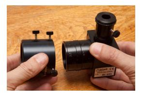
Assemble this part onto the Alpy 600 body - tighten firmly:
