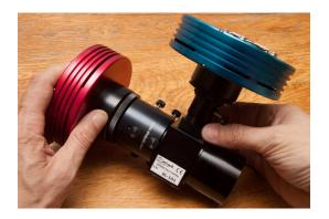
Take continuous images while turning the guiding optics. Try to maintain the camera orientation during this operation to make the image easier to read (it is not comfortable if the image is turning continuously). The slit image should become more and more focused. Eventually you should see it very sharp, and horizontal:
