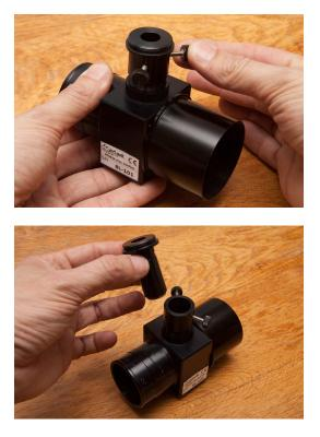
Mount the guiding camera on the guiding port, and tighten it firmly (the Atik Titan camera below has a Tmount thread - we've added a C-mount to T-mount adapter):
