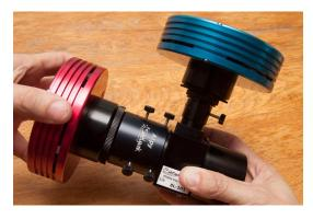
The optimal position is when the vignetting is minimal. When you've found it, tighten firmly the six knurled thumb screws.
