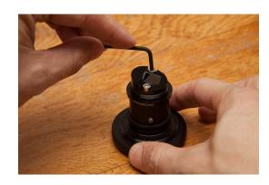
The nominal thickness (base to slit) of the standard and guider slit holders are identical (5mm). However, there is some manufacturing tolerance so you should check that the focus of the Alpy 600 is still correct (refer to the Alpy 600 user guide). From the spectroscope standpoint, the guided slit is the equivalent of the standard  $25\mu$ m slit (except the width is  $23\mu$ m with guiding module).
