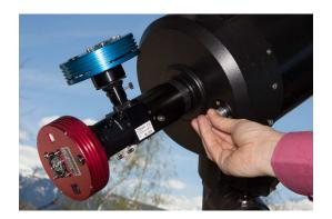
The focus of the slit comes from the guiding camera tuning (which should have been done on the bench). The focus of the object comes from the telescope tuning. When the instrument is ready, both slit & object must be focused in the guiding image.
