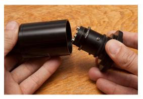
The Alpy 600 spectroscope has a removable slit holder. Remove the two screws, then the holder:
