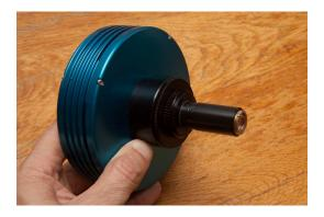
Re-assemble the guiding camera on the module (tighten a little bit the knurled thumb screws):
