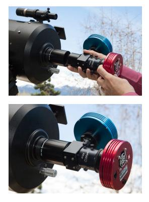
The orientation of the instrument on the telescope should be such that when you move the telescope along the Right Ascension (RA) axis, the image moves across the slit. This is only a question of comfort, but it is easier to center the star in the guiding image if the movements of the telescope are aligned with the axes of the guiding image.
