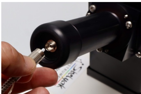
Figure 3.9: Connect the Fiber to the eShel III
