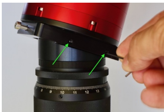
Figure 3.6: Mounting the camera to the eShel III lens
