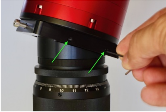
Figure 4.8: Release the dovetail screws, to allow the movement of the camera
