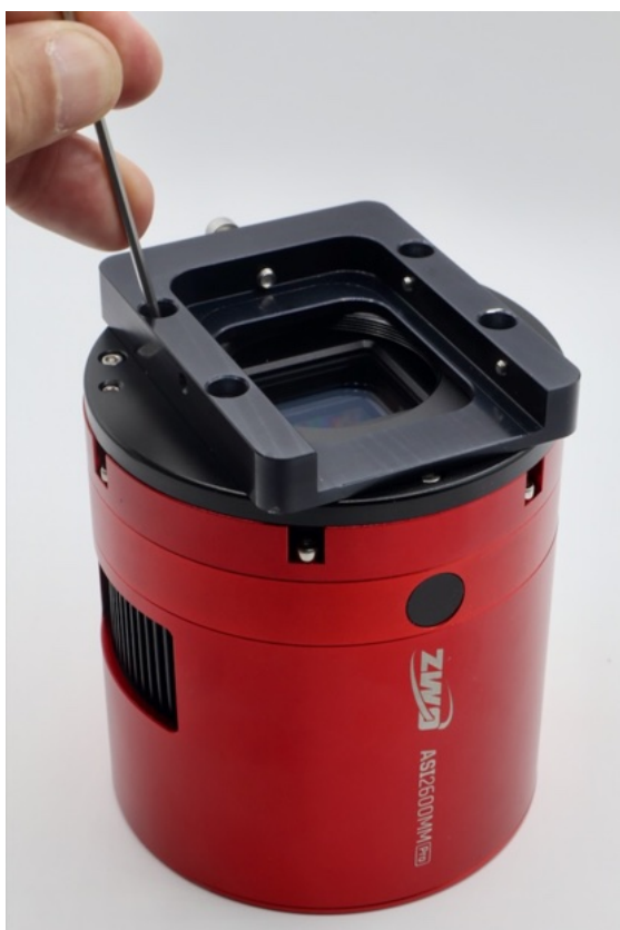
Figure 3.4: Attaching the camera plate
