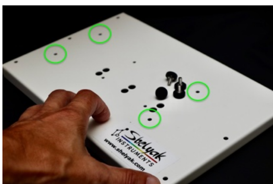
Figure 3.1: The base plate, before assembling. The green circles show the holes to put the screws in.
