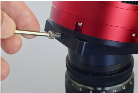
Figure 4.9: Release the dovetail screws, to allow the movement of the camera
