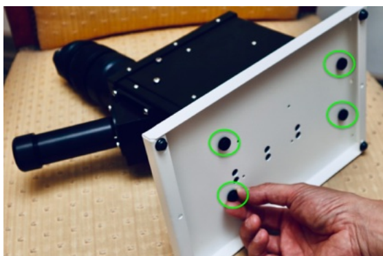
Figure 3.2: Attaching the Base plate to the eShel III. Green circles show the positions of the screws.
