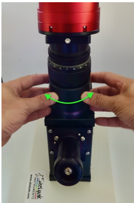
Figure 3.8: Rotate the lens to make sure the camera sensor is parallel to the eShel III chassis
