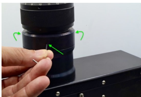
Figure 3.7: The screws to release before rotating the lens
