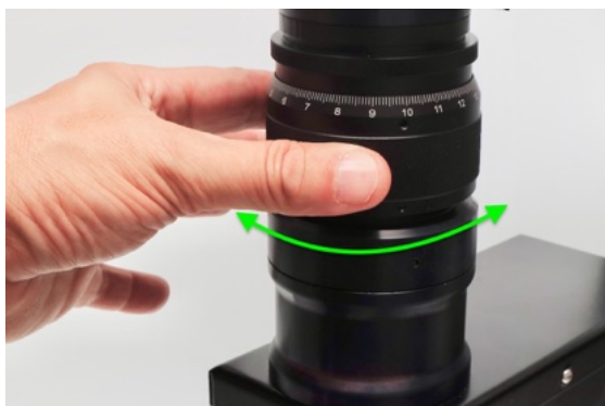
Figure 4.1: Rotate the ring to focus the image.
