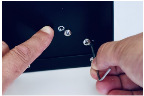
Figure 4.6: Release and tighten headless screws to center the spectrum in the image.
