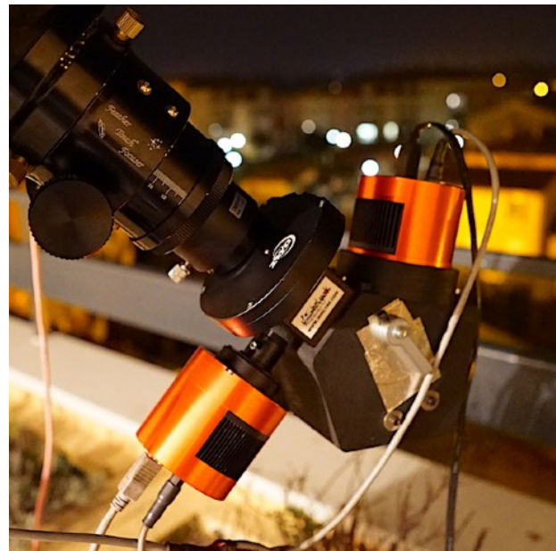
The red order filter is fixed into a filter wheel (ZWO).
